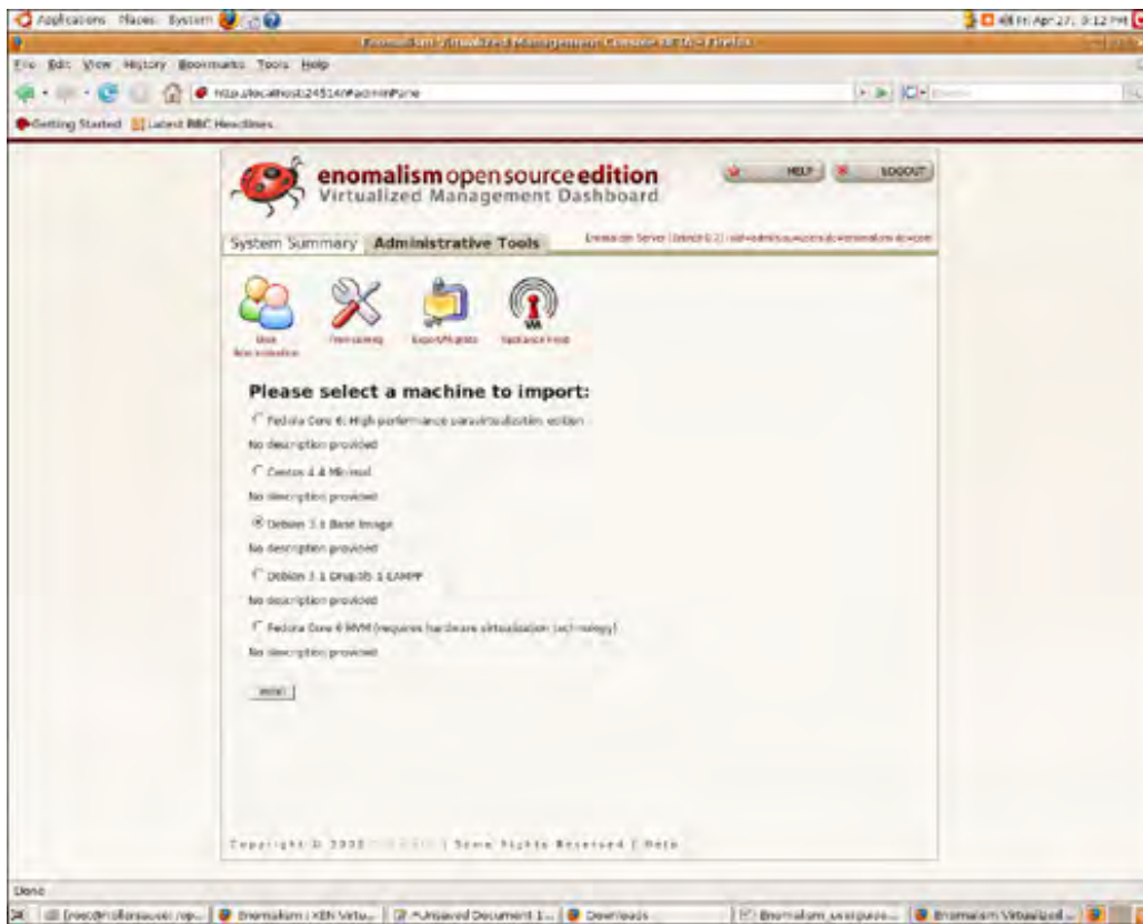
Figure 14.4 and Figure 14.5 illustrate the process of selecting and downloading a virtual machine image. After the image is downloaded, create a new virtual machine based on that image by choosing the destination Domain0 and a name for the new guest.
