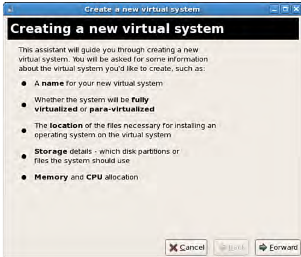
Figure 7.11. When creating a DomU, the Create a New Virtual System window appears.
